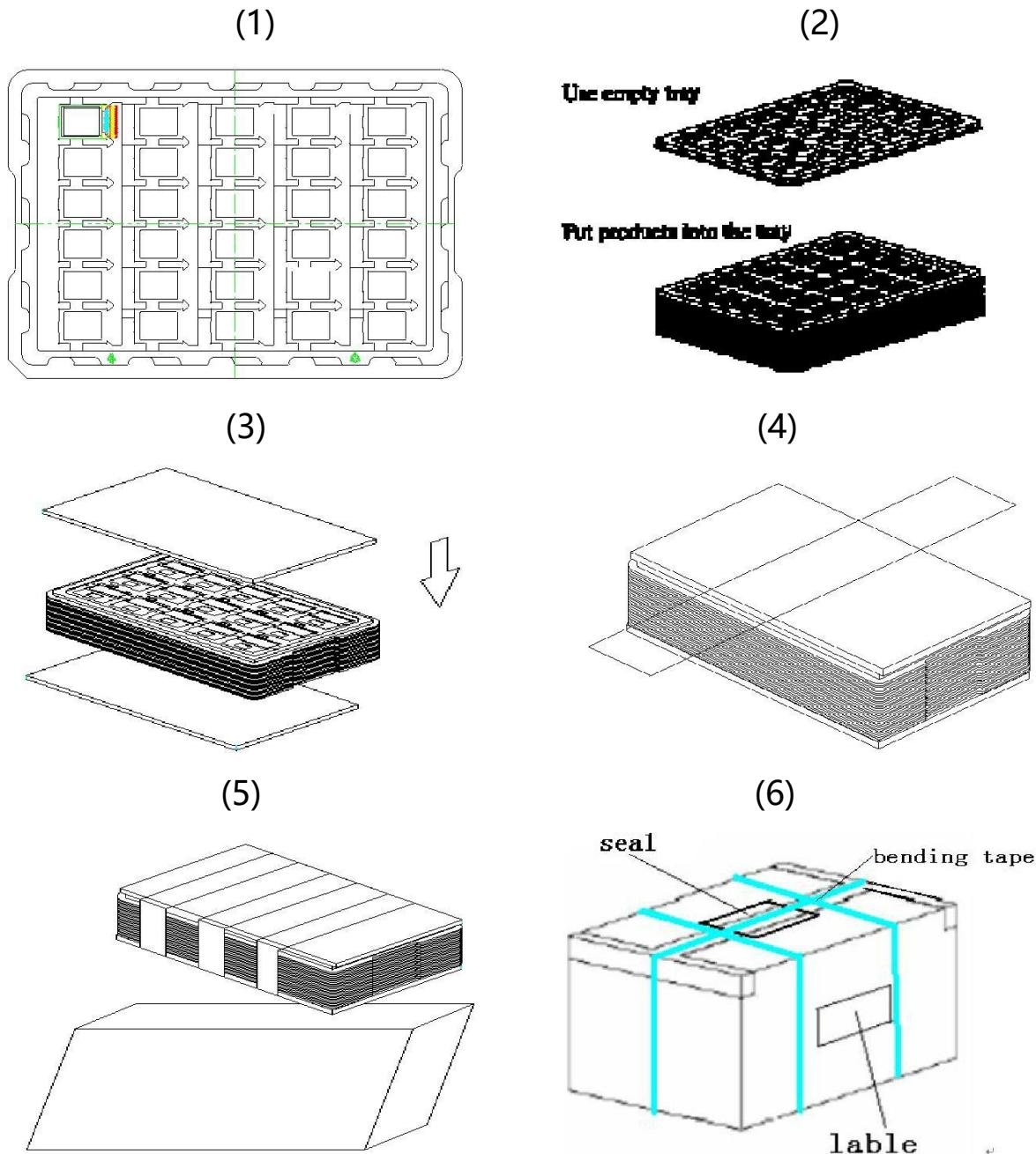
1. Put module into tray cavity. 把模块放进托盘.
